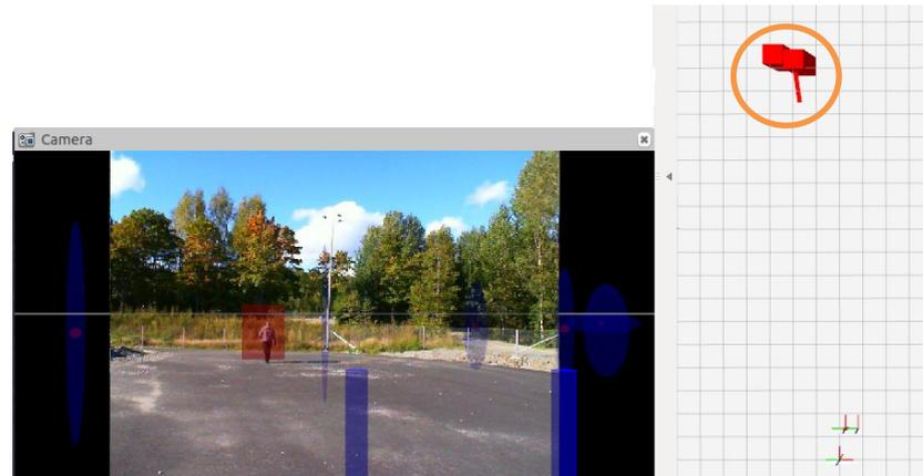
**Figure 16:** Test 3, Finding the Maximum distance till which a person is detected by the sensors.
